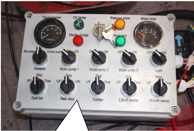
Main Control Box in Driver Cabin, which suggest fixing between seats
