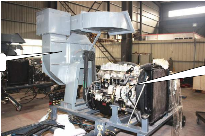
Auxiliary Engine Assembly: JMC brand 57kw
