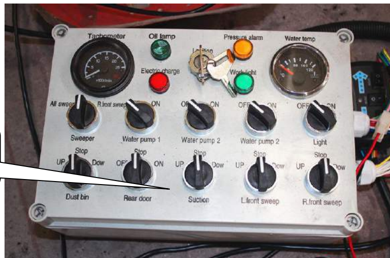
Control Assembly Main Control Box in Cabin
